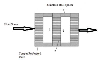
Figure 1 cross section of a matrix heat exchanger
