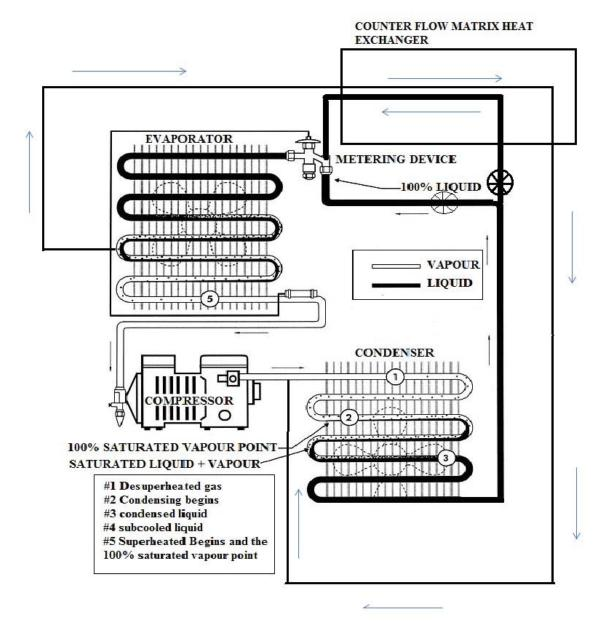
Figure 2 Proposed vapour compression refrigeration system using matrix heat exchanger
